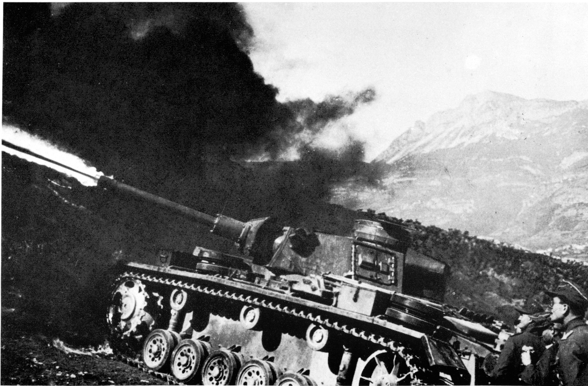
Here a Flammpanzer III of the 44th Infantry Division is seen. The burning oil capacity of 1,020 liters allowed eighty bursts of flame, each two to three seconds long. These vehicles, though, did not live up to the troops' expectations. For that reason, some of the Flammpanzer III tanks were soon (1943) rebuilt into normal battle tanks.
